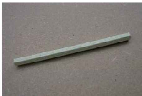
19-perf, slotted, rosette of GUDN propellant NZK5263
