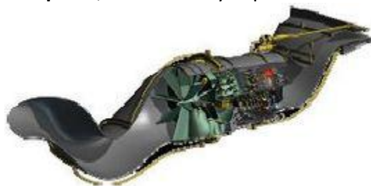
Cut-away view of a prospective ADVENT engine
