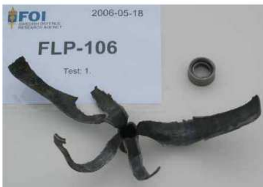
Figure 3. Results from the 25 mm detonation test, DN 25 [20].
